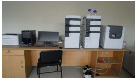
Fig: High Performance Liquid Chromatograph (HPLC) with Mass Spectrometer (MS) Detector
