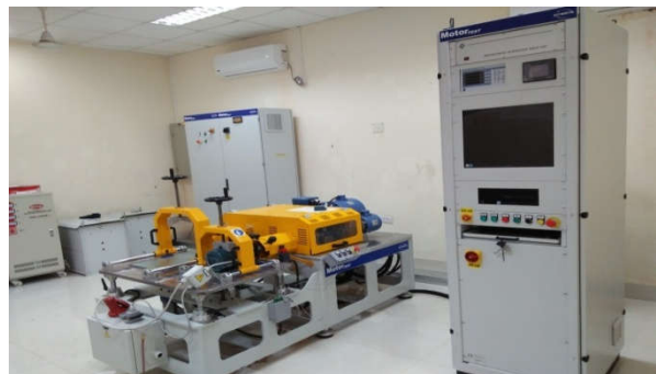
Fig: Motor Testing Unit ( 0.18kW to 10kW Electric Motor)
